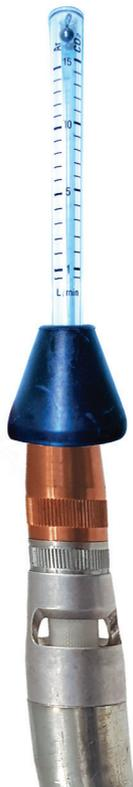
**Attention:** Poor gas protection leads to poor welding quality.
